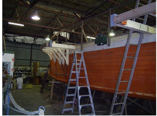
Curlip Rudder with Paddles ready to be mounted where the ladders are between the struts. The struts and the timber edge around them prevent the paddles being damaged by overhanging branches or jetties.
