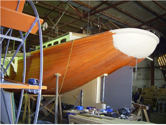
Curlip Rudder with Paddles ready to be mounted where the ladders are between the struts. The struts and the timber edge around them prevent the paddles being damaged by overhanging branches or jetties.
