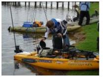
This photo shows the tank at the rear of the Hobie for storage of live fish prior to weigh in and the tall black rod at the rear is an electric anchor which can be raised and lowered to hold the craft in water between two and three metres deep. An interesting invention, particularly for waters like Lake Tyers where edges are muddy.
